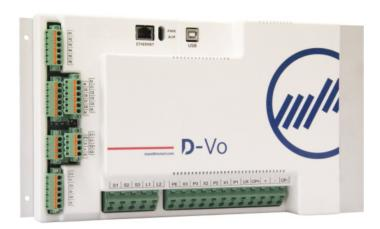
The new Digital Voltage Regulator D-Vo is an electronic microprocessor-based device which manages the operating electrical parameters of synchronous generators. The power supply to the exciter is through a PWM power stage.
